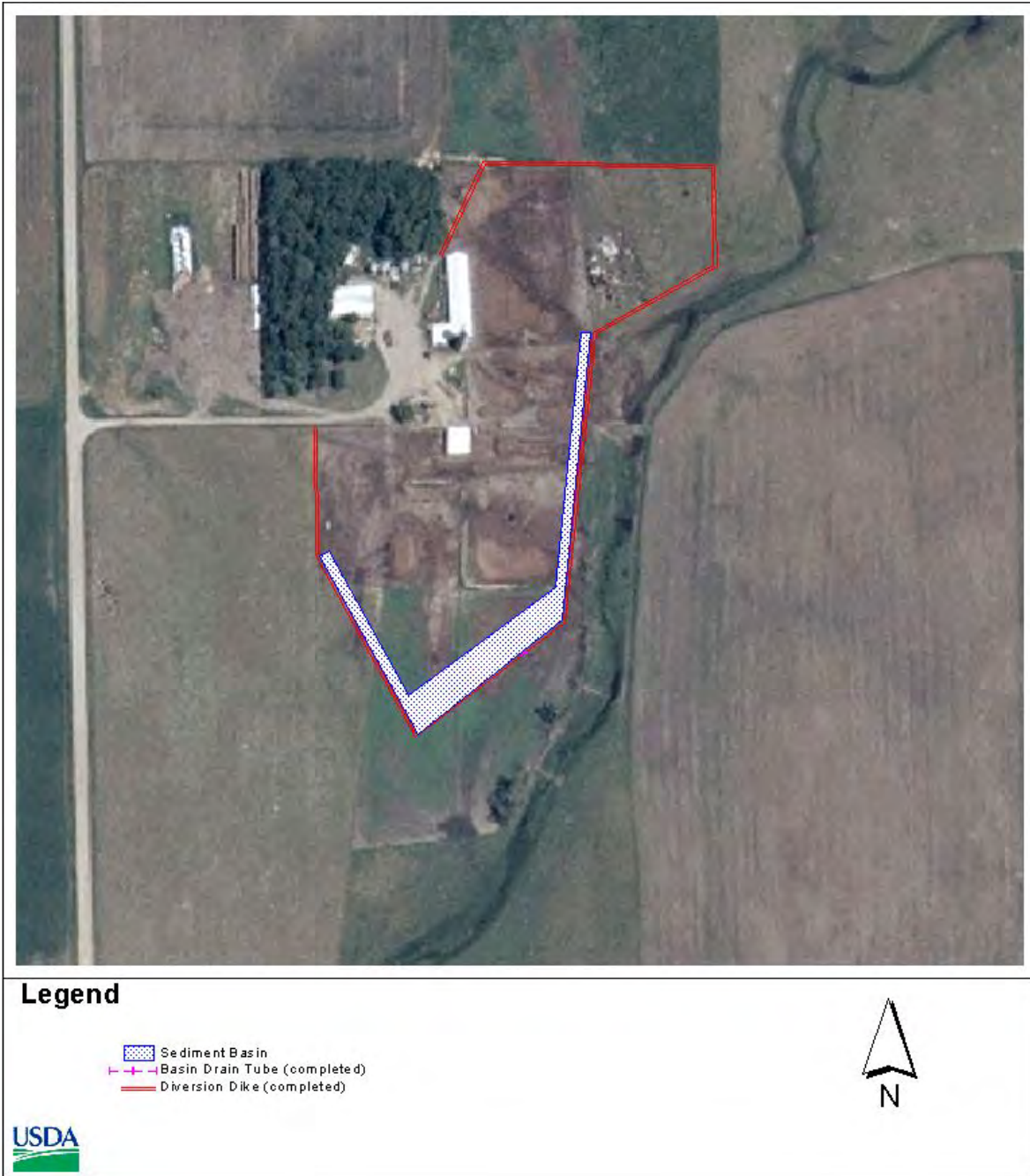
Figure 2. Clean Water Diversion System.
